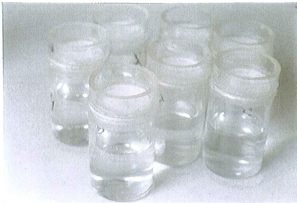
Fig.1: Preparation of the samples for the determination of water vapourpermeability
